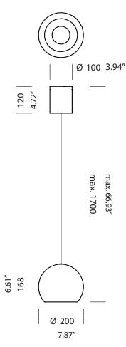
Installation note: Comes with a 4" backplate that mounts to a standard junction box
